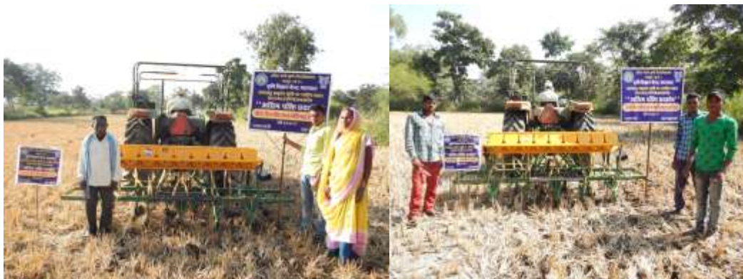
FLD on Zero till seed cum fertilizer drill for sowing of Mustard and wheat
